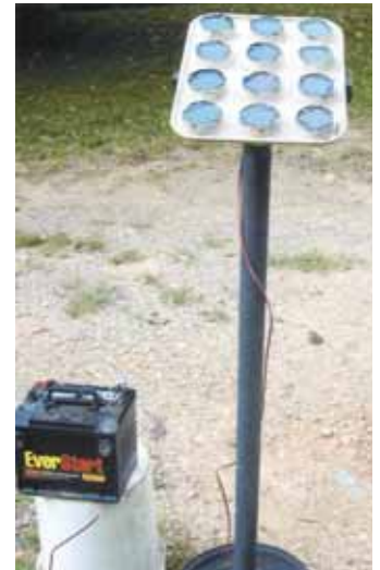
Eugene Taylor built this small solar panel, using a muffin pan and 12 small solar lights.
