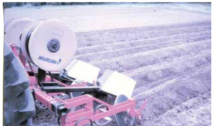
Rick Ratcliff gets raised beds ready for veggie planting with a potato hiller attachment originally designed to make trenches for planting spuds.
