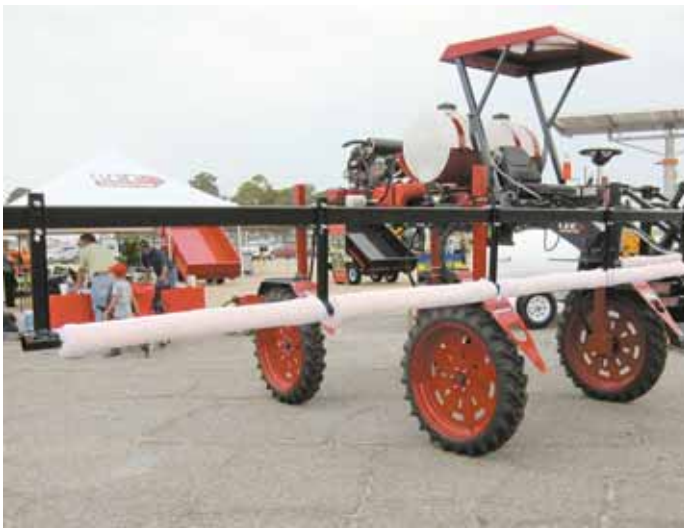
This high clearance, self-propelled “Lee Spider” was on display at the recent Sunbelt Ag Expo, equipped with a 30-ft. Smucker sponge wiper mounted on a toolbar.
