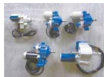
**Solar-powered system uses 24-volt motors to open and close roll-up sidewalls, maintaining the desired operating temperature inside greenhouse.**
