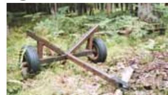
**Using sq. tubing he welded a tongue onto the angle iron, then welded a V-shaped log holder on top.**
