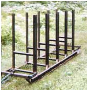
**Firewood-cutting rack is fitted with H-shaped uprights spaced 20 in. apart.**
