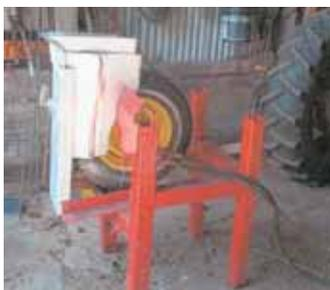
Larry Palmby built this walnut huller by mounting a wheel hub and tire on a metal frame (above). Homemade cracker (below) is fitted with a 10-in. long bolt that has a 4-bladed knife screwed onto the bottom.
