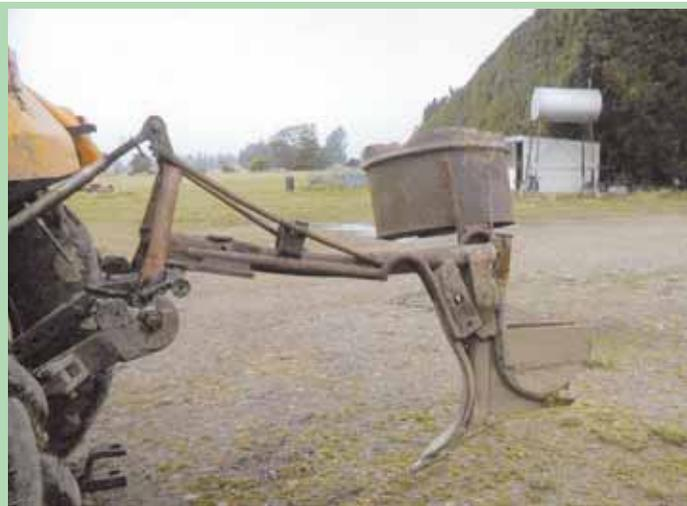
Home-built “knife” cuts a slot in the ground. As the tractor driver pulls the planter another person walks behind, placing trees in slot.
