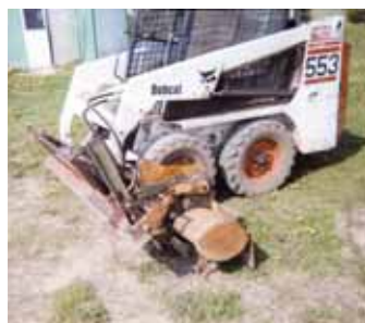
Tiller is belt-driven by an orbital motor off a fertilizer auger.
