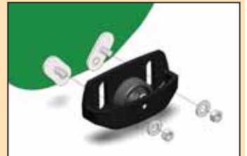
Roller-Skids replace snowblower's original factory skids. "The wheels roll easily on dry surfaces, and the skids take over on snow and ice," says inventor Bill Raftery.
