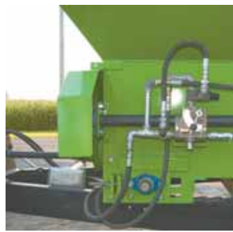
A hydraulic motor drives the gearbox and turns the shaft that drives the unloading chain. A variable hydraulic flow valve allows Lalonde to precisely change speeds.
