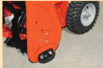
Roller-Skids replace snowblower's original factory skids. "The wheels roll easily on dry surfaces, and the skids take over on snow and ice," says inventor Bill Raftery.
