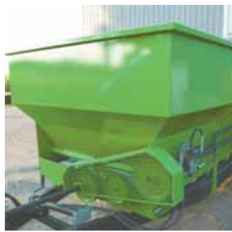
Steve Lalonde used parts from an old Massey Ferguson manure spreader to build this low-profile spreader for his poultry operation.
