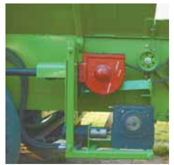
A hydraulic motor drives the gearbox and turns the shaft that drives the unloading chain. A variable hydraulic flow valve allows Lalonde to precisely change speeds.
