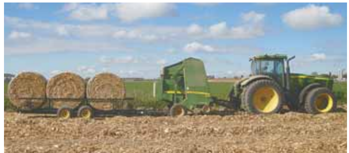
Randy Clark’s 35A Round Bale Accumulator trails directly behind a round baler and holds 3 bales as they’re discharged from the baler.
