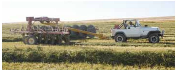
With clients up to 35 miles away, custom hay grower Luke Fuller uses a Jeep Wrangler to pull his hay rake. He fitted the Jeep with hydraulics to lift the rake for transport.
