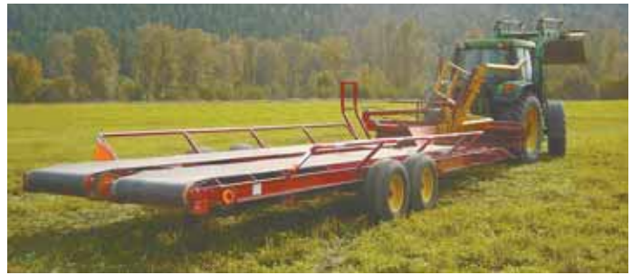
Bale wagon’s arms cradle and squeeze the bale, then lift and place it on a platform with a movable belt. Bales are never touched by sharp metal edges or a moving chain.
