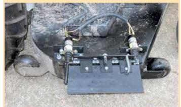
Powered drop-panel attachment drops down quickly to cover mower's chute opening at the touch of a button. Photo shows panel in the open position.
