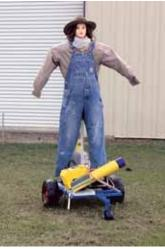
Scarecrow's metal frame holds a human form that swivels back and forth via an electric motor. Portable model can be fitted with a propane cannon.
