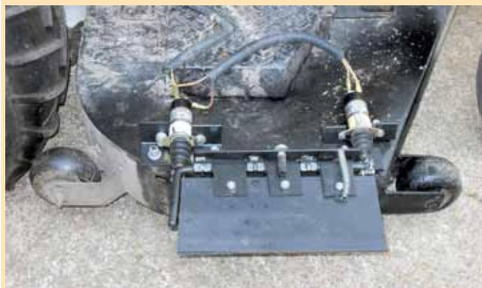
Powered drop-panel attachment drops down quickly to cover mower’s chute opening at the touch of a button. Photo shows panel in the open position.
