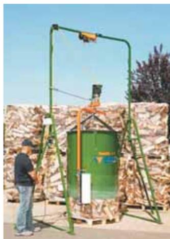
**PackFix mechanically creates a palletized bundle of firewood that's securely wrapped with plastic netting.**
