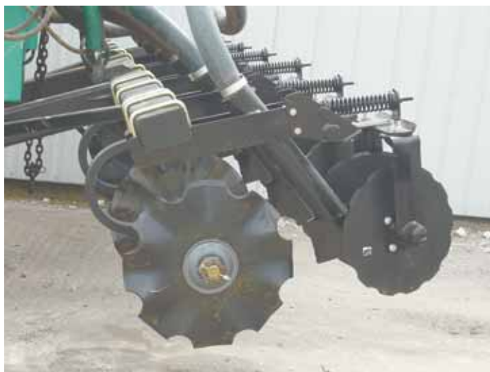
Vertical Till Injector clamps to toolbar mounted behind manure wagon and uses 22-in. wave notched blades, which are followed by V-shaped injectors.
