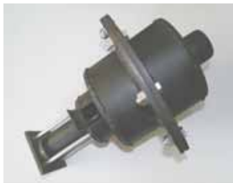
Pivot Flusher mounts by center pivot’s end gun. Each time the pivot stops and starts to pressurize, the water pressure automatically activates a complete system flush, then closes when irrigator begins to move.
