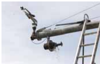
Pivot Flusher mounts by center pivot’s end gun. Each time the pivot stops and starts to pressurize, the water pressure automatically activates a complete system flush, then closes when irrigator begins to move.
