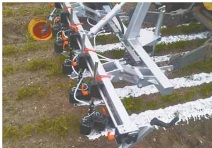
Weedintech’s Foamstream uses a combination of hot water, steam and foam to kill weeds on contact. The foam acts as a thermal blanket, trapping heat on the weeds.
