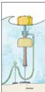
**Floating buoy rides the waves, driving underwater pump.**
