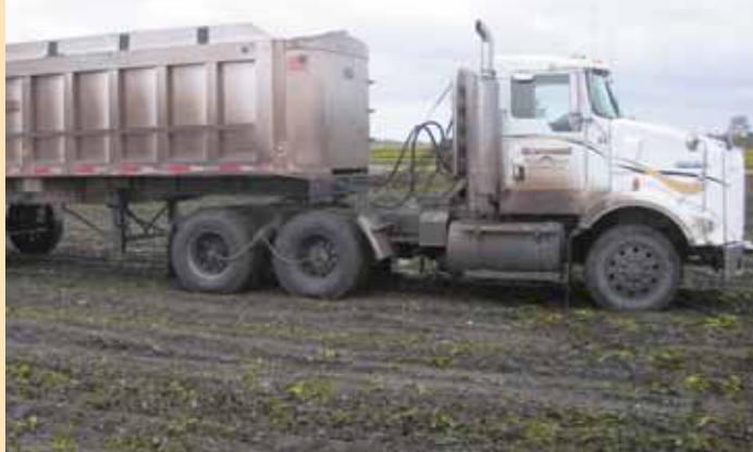
Air hoses attach to each drive wheel. Computerized system allows driver to inflate and deflate tires while the vehicle is in motion.
