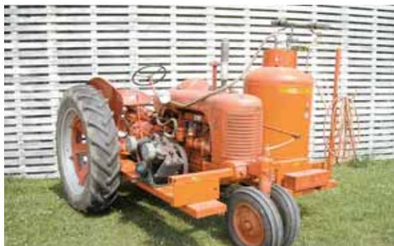
SC Case tractor belt-drives an air compressor on one side of tractor, which feeds air into a big 200-gal. tank on other side.
