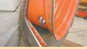
Tire monitor uses a sensor that mounts behind wheel rim, where it can't get knocked off.
