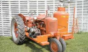
SC Case tractor beltdrives an air compressor on one side of tractor, which feeds air into a big 200-gal. tank on other side.
