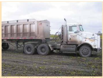
Air hoses attach to each drive wheel. Computerized system allows driver to inflate and deflate tires while the vehicle is in motion.
