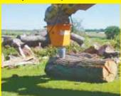
Our hands-free log splitter, designed for skid steer and mini excavators, is available in 3 different models that can split any log from 30 in. to 24 ft. long. All models operate off a hydraulic power head. The H.F. 100 can split a 30-in. long log of any diameter and sells for \$3.995.
