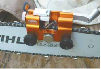
Timberline's crank-type chainsaw sharpener comes with a carbide cutter that rides the bar. The operator pulls the chain through to sharpen each tooth.
