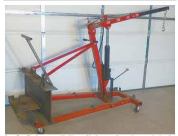
Steve Brouillard came up with this portable shop crane by turning a standard engine
