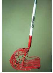
As scoop is pulled along the ground, the fruit is scooped up and held in the basket.
