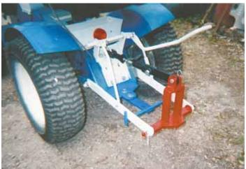
To make this 3-pt. mounted drawbar, Seltzer welded a length of rerod to a flat piece of steel that hooks onto the tractor's original 3-pt. hitch. The rerod supports the 3-pt.'s lower lift arms so they can't drop down too far.
