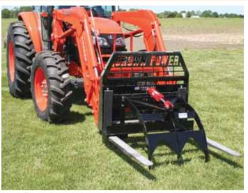
Add-A-Grapple comes with its own hydraulic cylinder and attaches to standard pallet forks with a screw-on lockdown clamp and a locking pin.
