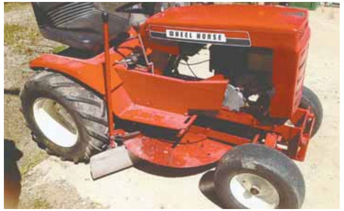
Wheel Horse “belly grader” is equipped with a 4-ft. grader blade that rotates on a circular steel platform and is hydraulically raised and lowered.
