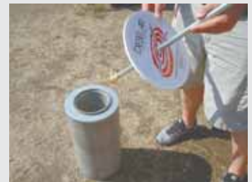
You simply insert rotary nozzle into filter with cover on top, and then slide it up and down to clean entire filter.
