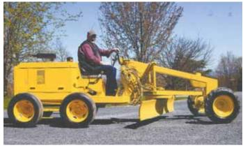
Jack Hockenberry built this 4-WD road grader that's equipped with a 6 1/2-ft. wide blade that can be moved in any direction.
