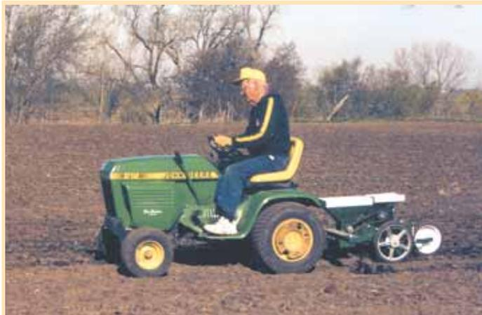
John Beran uses this one-row planter on his Deere 212 garden tractor. A pair of ground-driven rubber wheels are used to chain-drive fertilizer and seed metering units.
