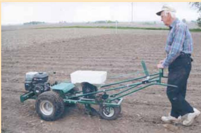
He used the transaxle and rear wheels from a Massey-Ferguson garden tractor and a 6 1/2 Briggs & Stratton engine to build this self-propelled, walk-behind planter.
