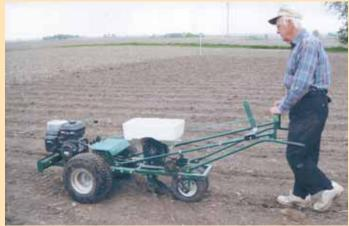
He used the transaxle and rear wheels from a Massey-Ferguson garden tractor and a 6 1/2 Briggs & Stratton engine to build this self-propelled, walk-behind planter.
