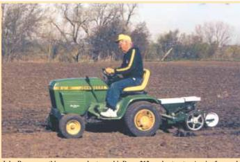
John Beran uses this one-row planter on his Deere 212 garden tractor. A pair of grounddriven rubber wheels are used to chain-drive fertilizer and seed metering units
