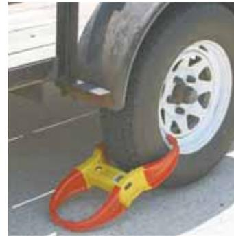
Wheel lock clamps onto wheels from 12 to 20 in. dia.
