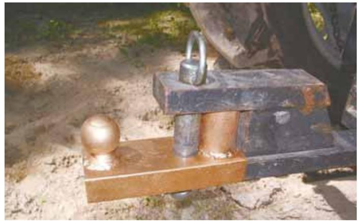
Heavy-duty adapter slips over drawbar to tow ball hitch trailers.
