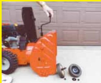
raise and lower the shoes automatically. A 9/16-in. socket is welded to the crank and fits over a nut welded on top of a 3/8-in. threaded redi rod. The rod runs down through blocks made from 1-in. sq. bar stock that I bolted onto one side of the blower housing. I had to do some cutting, drilling, tapping and welding to make the various parts.
