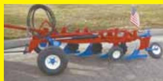
a good job of plowing, too. It's equipped with four 6 1/2-in. tall moldboards off an old David Bradley moldboard plow. The moldboards were individual units when I got them, so I welded together a frame to mount them on.
