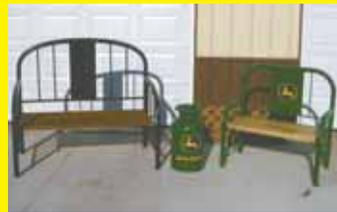
I make nice looking "bed benches" out of the metal headboards and footboards off old beds. I cut the footboard into two halves and then weld them onto the headboard to make the bench's sides. A 2 by 12-in. board serves as the seat. (Craig Wegner, 4122 Cherry Ave., Hawarden, Iowa 51023)
