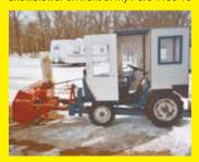
hp diesel tractor with a home-built cab. I installed a home-built frame under the tractor and ran a driveshaft from the rear pto up to the snowblower. I had to reverse the pto drive to match the snowblower's auger drive.
