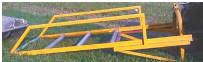
Russell Whitworth built this tractor-mounted boat hauler out of an old 3-pt. mounted sprayer. The boat rolls up on a series of 2-in. dia. plastic pipes spaced 1 ft. apart.
