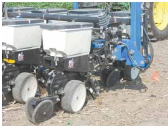
Becks Hybrids used a custom-built Kinze 8-row planter to research the concept of planting 2 different hybrids in a field at the same time.
