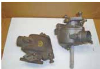
**Carburetors come in looking like the one on the left and go out looking like the one on the right.**
