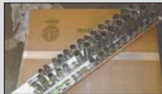
strips onto a 2-ft. long, 4-in. wide piece of kitchen countertop. I keep a 6 and 12-point socket next to each socket size.
