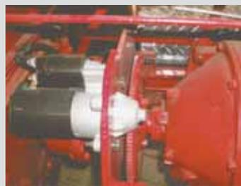
tractor. The ring gear is from a Ford Taurus and the starter is a Ford marine starter, which I used because it turns in the same direction as the crankshaft on the tractor's engine."
