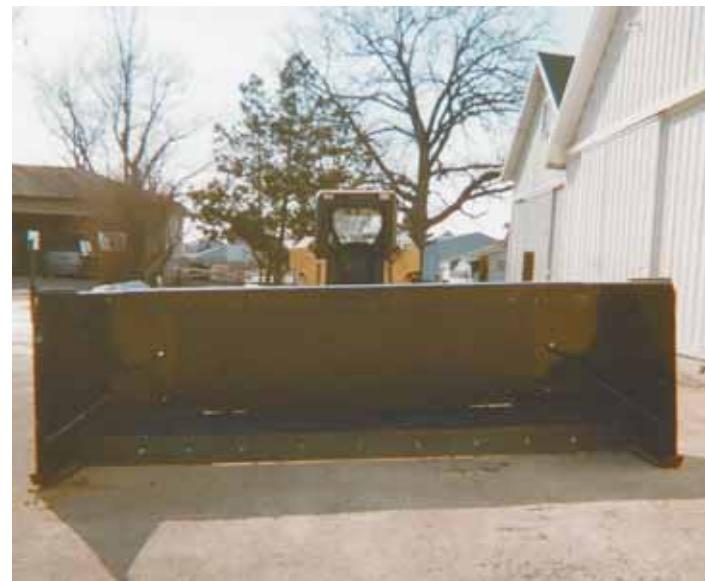
Roy Viel turned an old 20-ft. wide Deere grain platform into this skid loader-mounted snow blade. "It works just as good as a commercial rig," he says.
