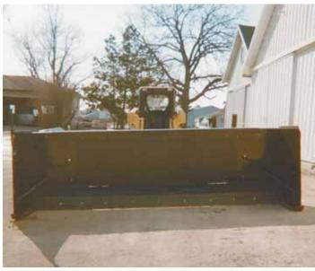
Roy Viel turned an old 20-ft. wide Deere grain platform into this skid loader-mounted snow blade. "It works just as good as a commercial rig," he says.
