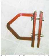
Bucket-mounted puller consists of a pair of steel plates and a clevis bar that's welded onto one of them.
