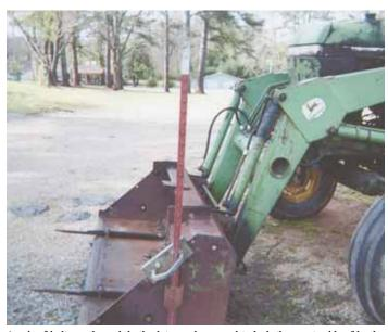
A pair of bolts go through both plates and are used to lock them onto side of loader bucket. Webb lets the bucket down over post, then raises the bucket to grab it.
