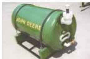
**Auxiliary tank rests on a pair of wooden blocks bolted to an angle iron frame (left). A 12-volt pump that runs off the tractor battery is used to operate the system.**
