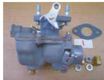
**Mike Finch restores Farmall Cub and Cub Lo-Boy carburetors to "better than new" condition. Photo shows new choke shaft and lever with cork top-to-bowl gasket.**
