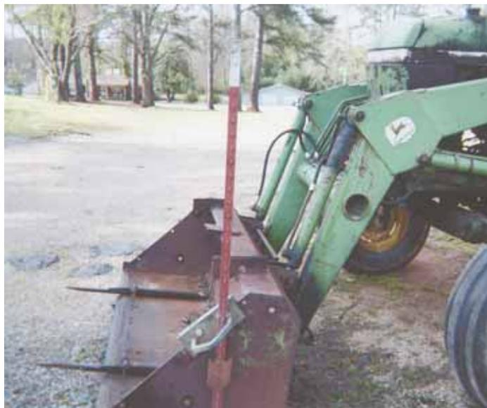
**A pair of bolts go through both plates and are used to lock them onto side of loader bucket. Webb lets the bucket down over post, then raises the bucket to grab it.**
