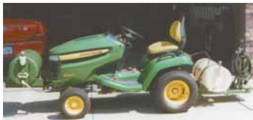
**Jim Rotter converted his Deere X540 garden tractor into a self-propelled mini spray rig complete with a 5-ft. boom, a hand nozzle, and an auxiliary tank on front.**
