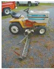
Figuring out how to mount mower with full hydraulic lift was quite a challenge, says DeLooza.
