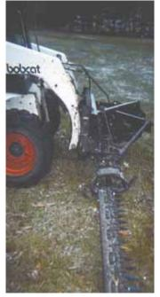
Ron Schneider adapted an old New Idea sickle mower to use on his skid loader.
