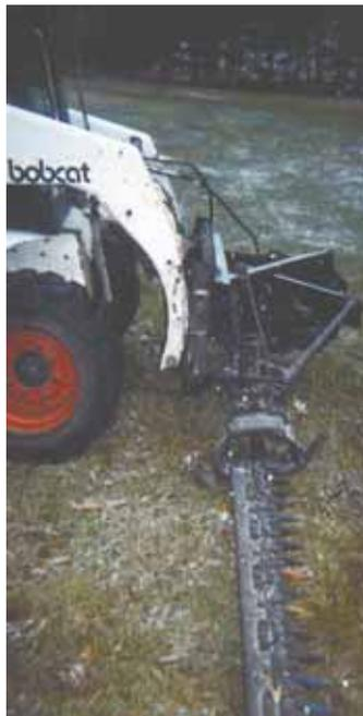
**Ron Schneider adapted an old New Idea sickle mower to use on his skid loader.**
