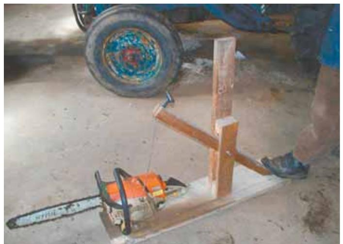
Chainsaw is secured to wood frame. Saw's pull cord slips through a notch at end of wooden lever. Quickly pushing down on lever with foot pulls cord to start saw.
