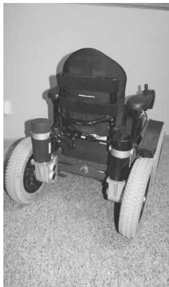
Sullivan bought 4 quality wheels off eBay and uses 4 motors to run them independently. To reduce weight, he made a compact aluminum frame just big enough to hold the motors and wheels.
