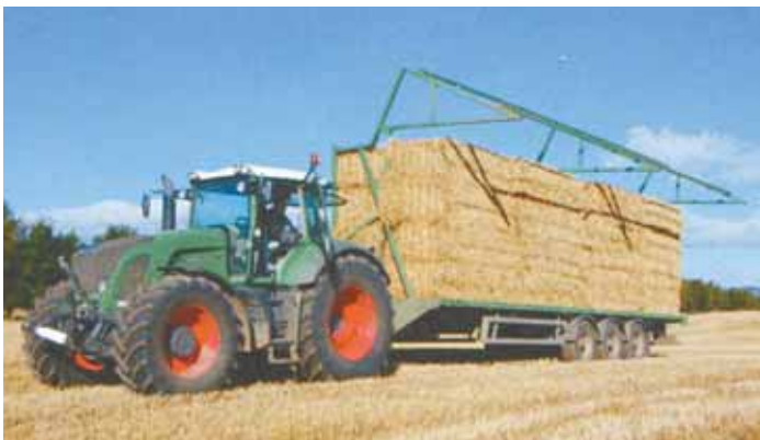
Trailer holds up to 32 big square bales and is equipped with a hydraulic-operated clamshell, which opens for loading and then closes down on one side of trailer for transport.
