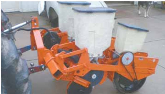
Doug Strouse converted a 6-row, pull-type Allis Chalmers planter into this 2-row, 3-pt. mounted model.
