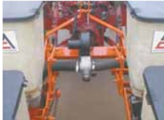
He chopped the planter toolbar back to about 6 ft., enough for 2 planters on 30-in. rows (above). He also fabricated a 3-pt. hitch for it.
