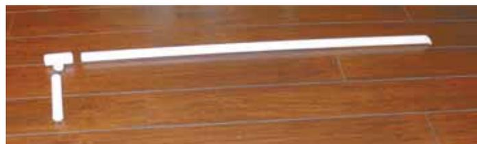
Eddie Rowland uses a hollow pvc “cane” to deliver poison bait into mole tunnels.
