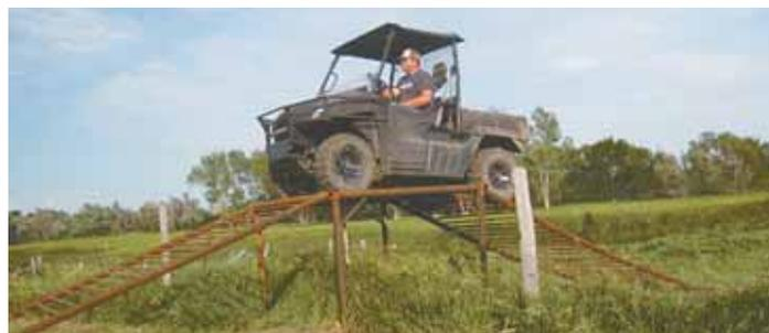
Drive-over gate comes with a 5-ft. long table and two 14-ft. long, 6-ft. wide ramps that bolt onto table. Bolts run through sleeves, allowing ramps to flex up or down.
