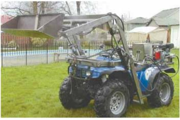
Heavy-duty EarthMover ATV loader has a 60-in. lift height and a capacity of 500 lbs. It's operated by a rear-mounted, 7 1/2 hp hydraulic power pack.
