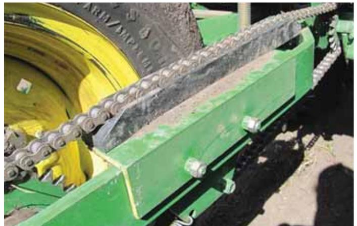
**"Tire Saver" kit is designed to stop swing arm and tire damage on Deere 7100, 7300 and 1710 3-pt. mounted corn planters. Chain is held in place by a bolt-on plastic guide.**
