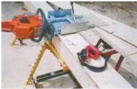
Attachment bolts onto chainsaw bar, allowing Rodler to make wood siding and other beveled wood products.
