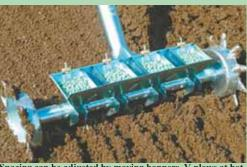
Spacing can be adjusted by moving hoppers. V-plows at bottom of each hopper create row openings as seeder is pulled toward operator
