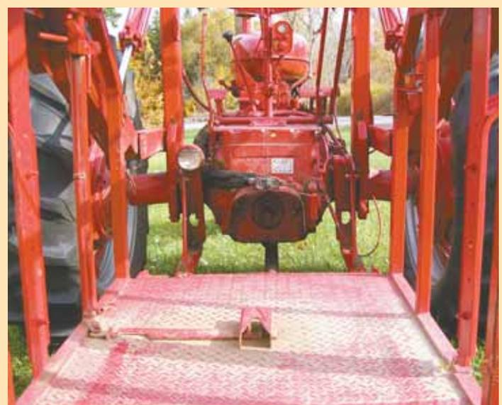
Repka rolls his wheelchair onto lift deck and locks chair in place to a wheelchair locking system. A toggle switch is used to raise the lift.
