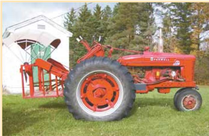
Quadriplegic Mark Repka designed this covered handicapped lift for his Farmall. It's bolted to rear axle and operated by a separate motor, battery and hydraulic system.
