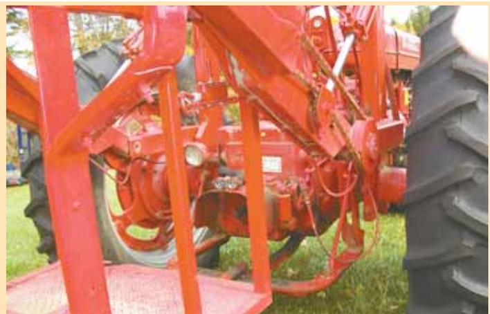
Besides removing the tractor's seat and moving the battery, modifications were made to the clutch and brakes, and the steering wheel was extended.
