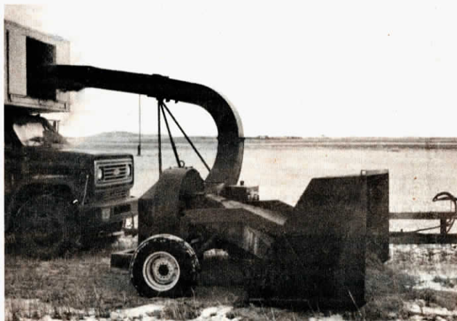
Vacuum chaff harvester sucks up piles of chaff and blows them into trailing truck.
