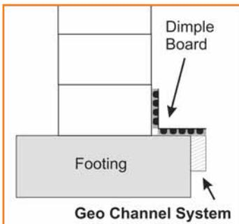
This system has been proven over the last 25 yrs. in most professional football fields. Installed without rock and it doesn't plug. In a basement the company suggests using a little 3/8" pea rock to give you more collection surface so you can flow more water. It requires a lot less labor than regular drain tile systems. Labor is the biggest cost factor in drain tile systems. The Geo channel system uses less materials, also less dirt and broken up concrete is handled, resulting in less cost.
