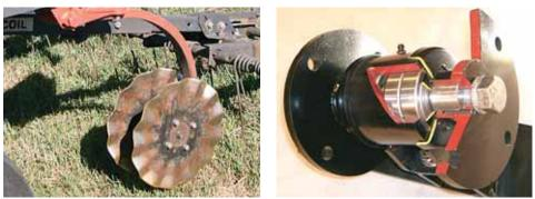
Coulter kit includes 18-in., 13-wave boron "earthenharden" coulter blades (left). Kit (right) is now fitted with 4 bearings to make it even more heavy-duty. Works in wheat stubble and corn stalks. Cuts up trash so you can plant days earlier.
