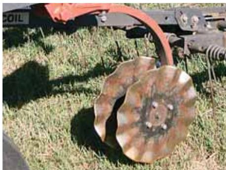
**Coulter kit includes 18-in., 13-wave boron "earthenharder" coulters blades (left). Kit (right) is now fitted with 4 bearings to make it even more heavy-duty. Works in wheat stubble and corn stalks. Cuts up trash so you can plant days earlier.**
