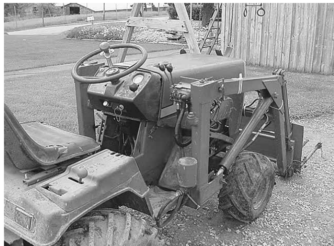
Loader's 2 1/4-in. dia. lift cylinders came off a New Idea hay baler.
