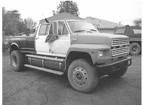
Doug Fry converted his 1987 Ford F-800 into this 210 hp dually pickup equipped with a crew cab. It's fitted with twin 115-gal. fuel tanks.
