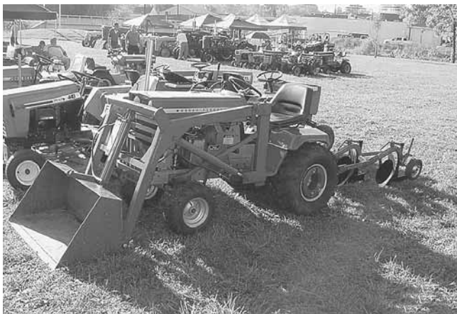
Daniel Perkins built this front-end loader from scratch for his Massey Ferguson 1650 garden tractor.
