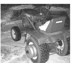
A wide variety of adapter kits are available, allowing you to mount weights on a tractor's drive wheels or on the front, back or sides of the tractor.
