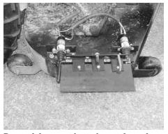
Powered drop-panel attachment drops down quickly to cover mower's chute opening at the touch of a button. Photo shows panel in the open position.
